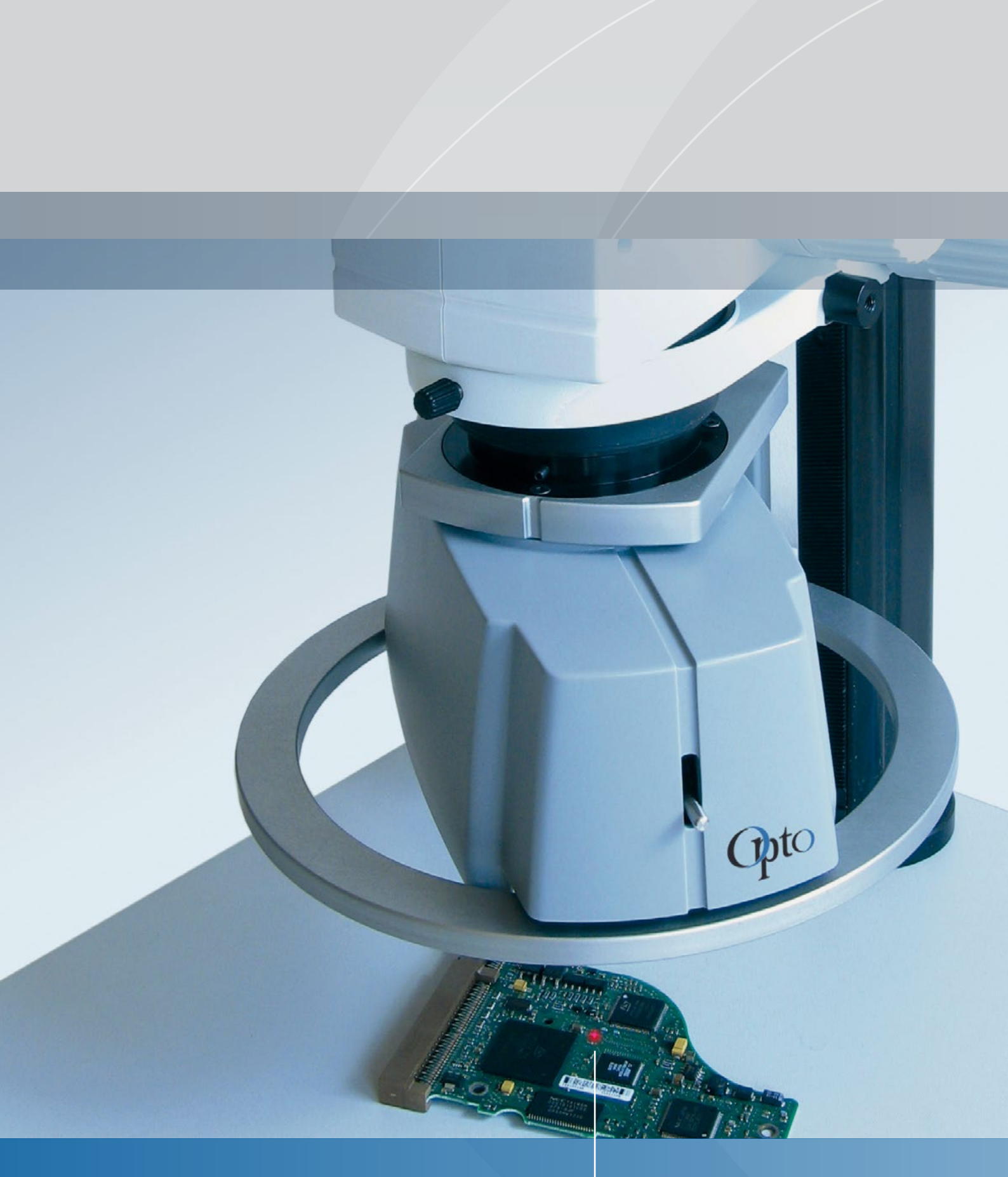
LED-pointer in oblique view for finding actual position
