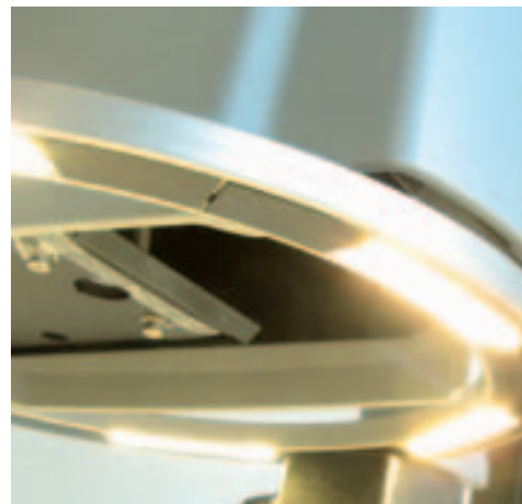
Assuring Perfect Image Quality: Integrated Objective and LED-Ring Light
