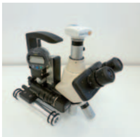
Optional Height Gauge enables precision measurement of layer thickness
