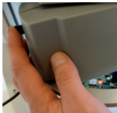
LED-Spot indicating the centre of the oblique field of view
