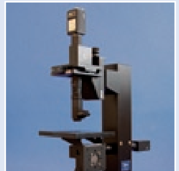
Top and Bottom Microscope System for Wafer alignment
